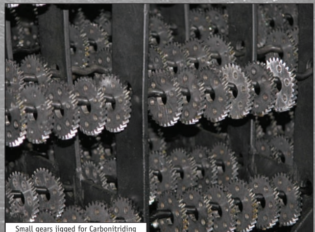
Small gears jigged for Carbonitriding
