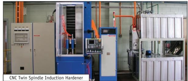
CNC Twin Spindle Induction Hardener
