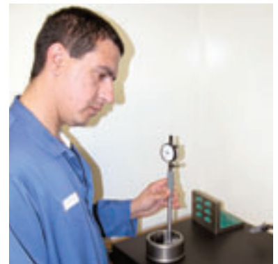
Terry Sassman (Quality Controller) checking the bore diameter of a component
